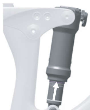
Figure 106: Moving the O-ring on the rear frame damper
