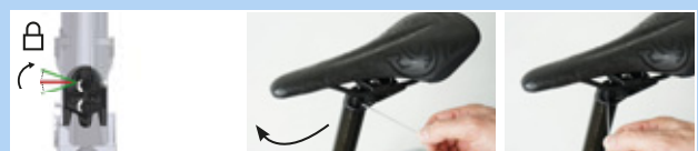
Figure 209: Closing the height adjustment
