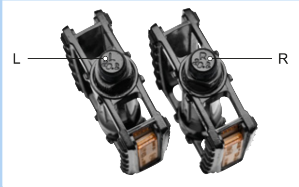
Figure 58: Example of markings on pedals
