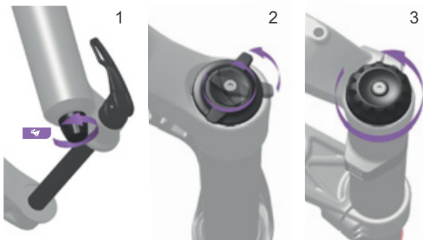
Figure 101: Opening the rebound damper (1) and compression adjuster (2 and 3)
