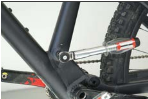
Figure 65: Tightening the seat post axle
