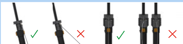
Figure 199: Correct and incorrect Bowden cable
