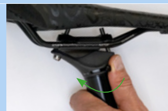
Figure 228: Closing the height adjustment
