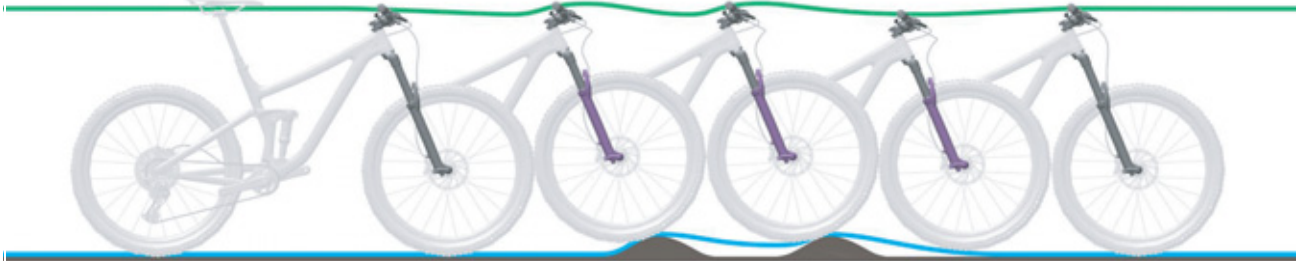
Figure 236: Suspension fork rebounding too slowly
