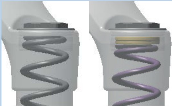
Figure 91: Screwing and unscrewing the preload adjustment ring
