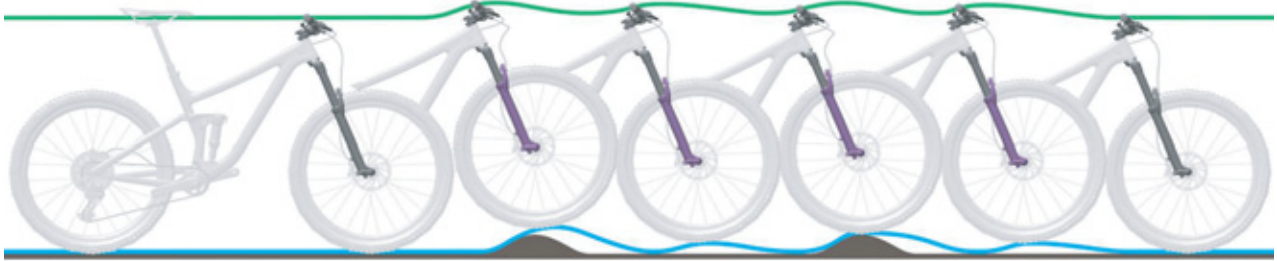
Figure 234: Suspension fork rebounding too quickly
