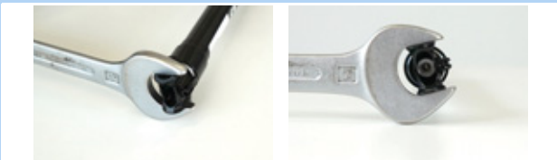
Figure 193: Securing against twisting
