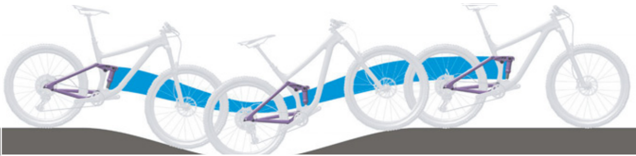
Figure 246: Excessively soft suspension in the rear frame damper on hilly terrain
