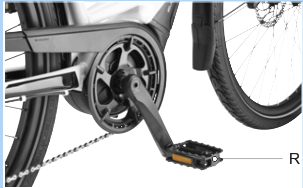
Figure 60: R-pedal in the right-hand crank arm
