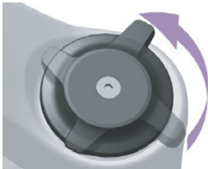
Figure 150: Changing compression adjuster to a softer setting
