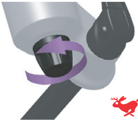
Figure 237: Turning the rebound screw damper towards hare symbol
