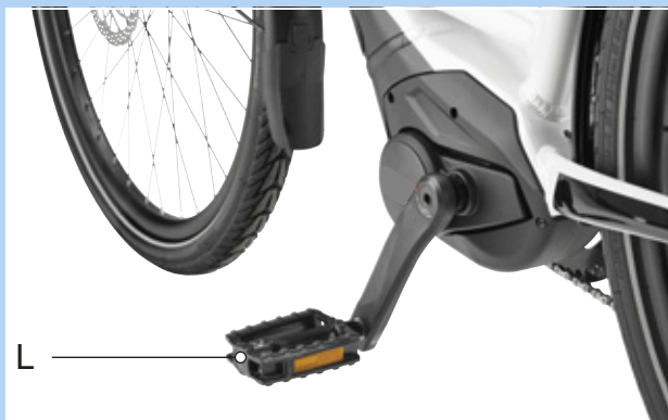
Figure 59: L-pedal in the left-hand crank arm
