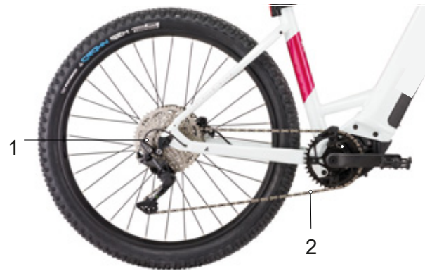
Figure 36: Chain drive with derailleur gears
