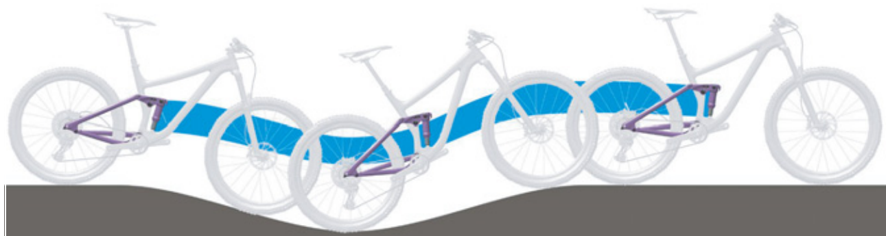
Figure 20: Optimum rear frame damper ride performance on hilly terrain
