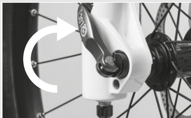
Figure 41: Closing the quick release
