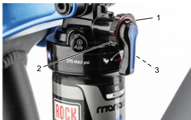
Figure 80: Setting the rebound damper strength on the rear frame damper setting wheel (1)
