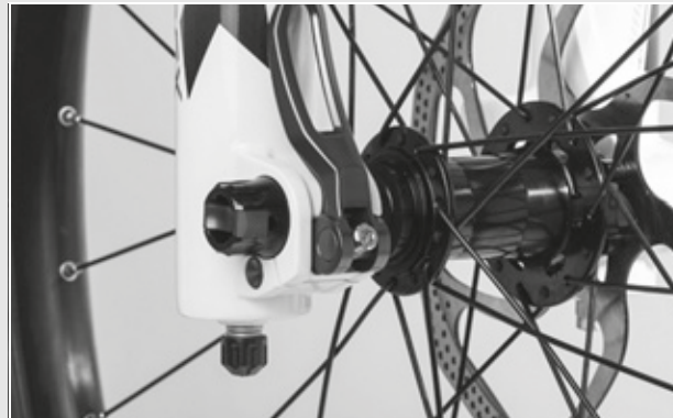
Figure 36: Perfect position for the clamping lever
