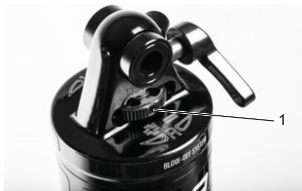
Figure 62: Suntour rebound adjuster wheel (1) on the rear frame damper
