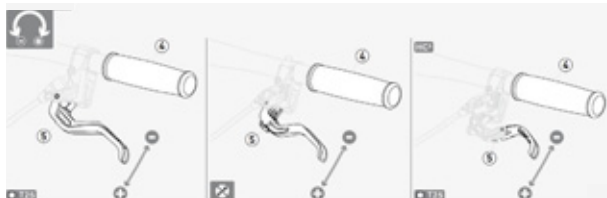
Figure 56: Setting the grip distance on a Magura disc brake lever
