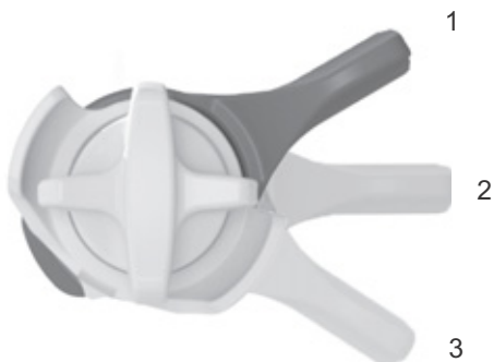
Figure 78: FOX compression damping adjustment on the rear frame damper with OPEN (1), MEDIUM (2) and HARD (3) positions
