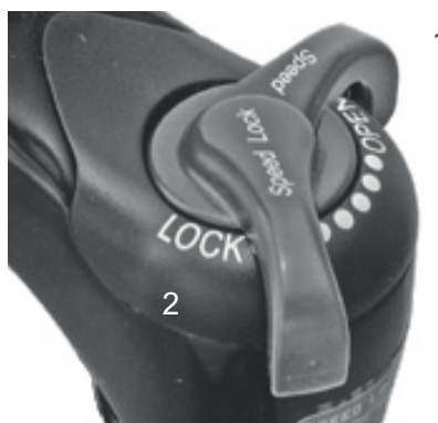
Figure 74: Suntour compression damping adjustment with OPEN (1) and LOCK (2) positions
