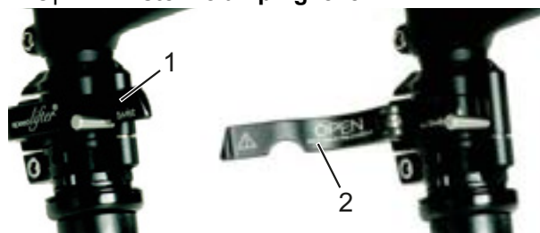
Figure 52: Open (2) and closed (1) stem clamping lever; by.schulz speedlifter used as an example
